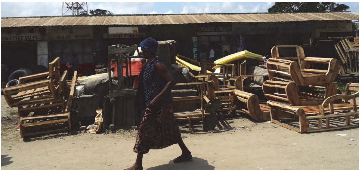
Figure 24. Wooden frames for lounge furniture that will later be covered and stuffed. These have been made by one of many entrepreneurs in the Bombolulu area, Mombasa where wooden pallets used to transport industrially packed products are available at low costs near this major East African port. Photo: A.B. Cunningham.
