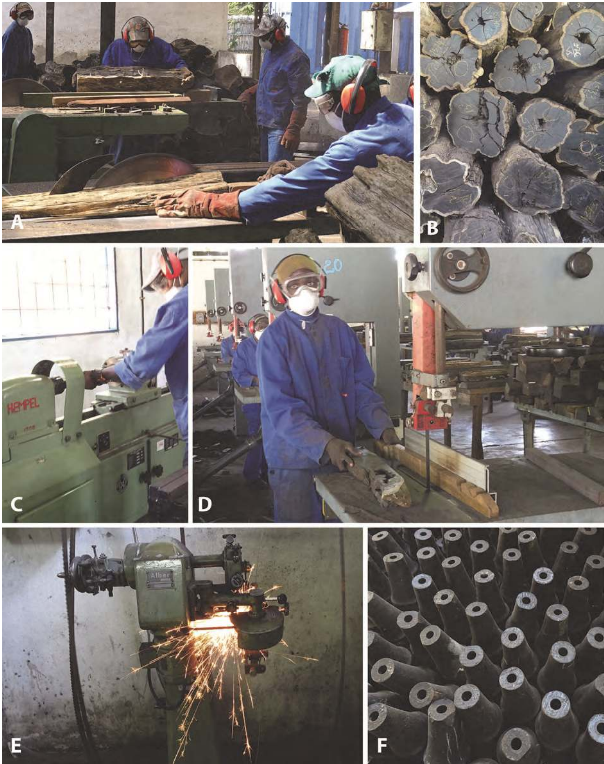
Figure 30. Mpingo Madeiras Lda.: creating employment and adding value after investing in training, equipment to produce world-class export products in remote northern Mozambique. A. Sawing D. melanoxylon into useable blocks, showing safety gear. B. Stacked logs of D. melanoxylon before processing into blanks for the world's best wood-wind instruments. C. Precision equipment for drilling through the centre of locally turned clarinet and oboe blanks. D. Use of band-saws to minimize the width of cuts and maximise wood use. E. Investment in an automatic band-saw sharpening machine. F. Stacked sections of clarinet blanks. Photos: A.B. Cunningham.
